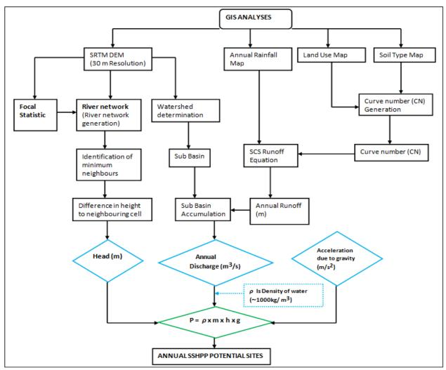
Fig. 2 Flow chart showing Research Methodology for Annual Hydropower Estimation.
