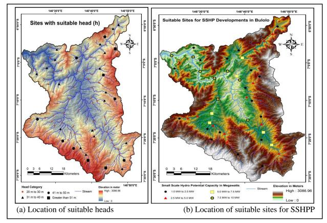
Fig. 7 (a) Location of suitable heads. (b) Location of suitable sites for SSHPP
