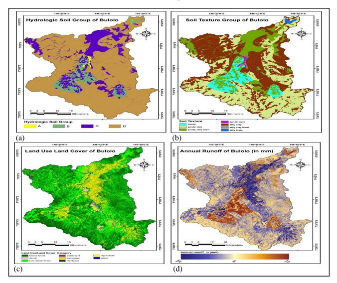
*Fig.6* Input maps for discharge. (a) Hydrologic Soil Group (b) Soil Texture Group (c) Land Use/Land Cover (d) Annual Runoff in mm.
