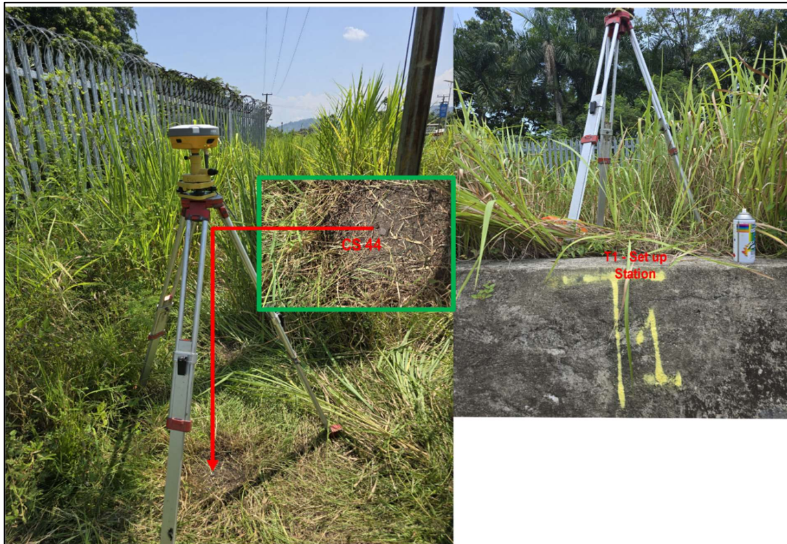
Fig. 3 Data collections by GNSS GPS (Global Positioning System)
