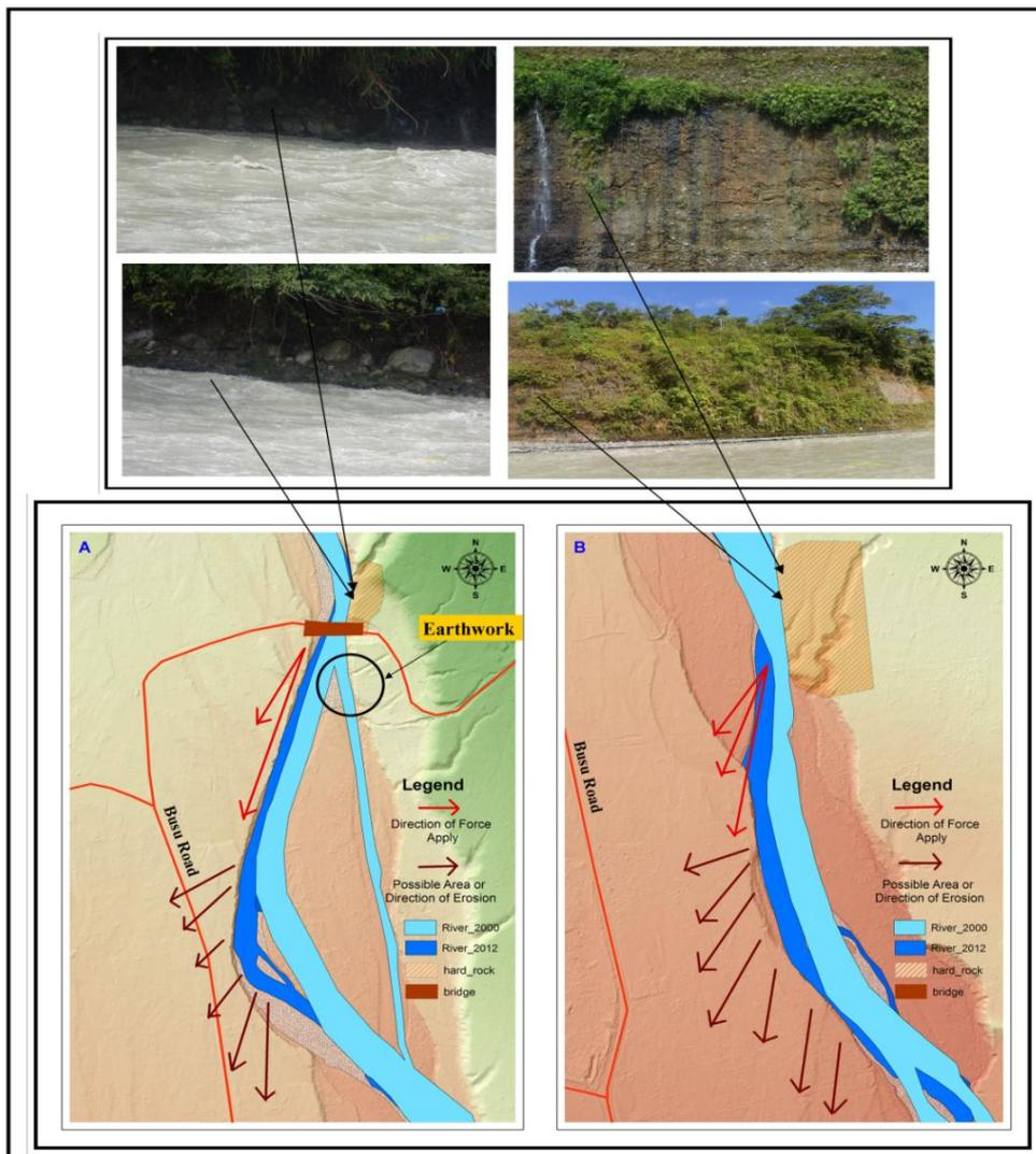
Figure 5: Possible direction of river force and erosion (Map A-LC1 & Map B-LC2)
